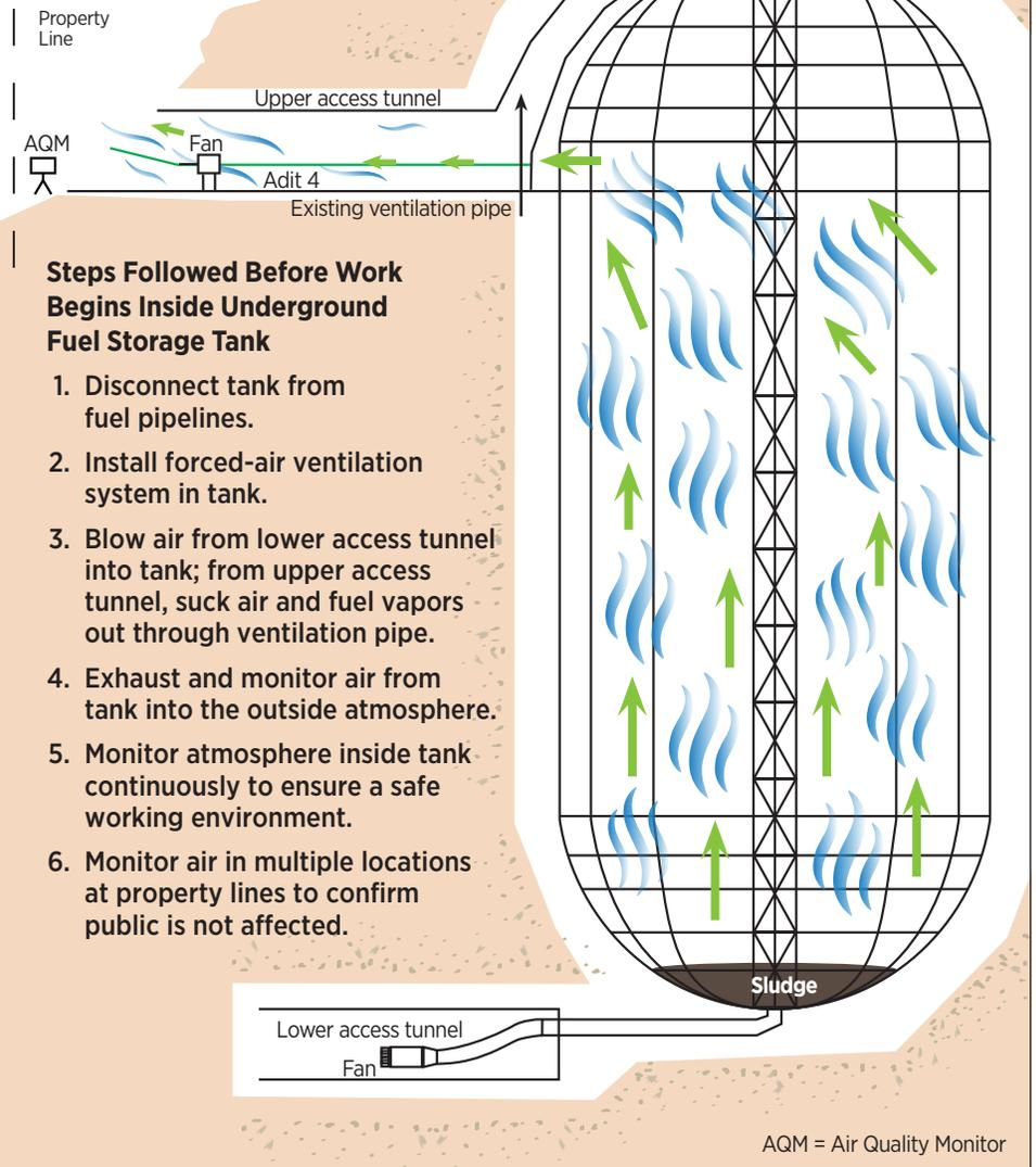
**Ventilating large underground fuel storage tanks is a crucial safety measure taken before any cleaning or repair procedure begins. The safety of personnel, the community, and the environment are paramount during this process.**
